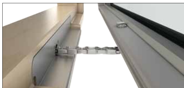
Electric opener for remote operation. For VELFAC 201, 203, 207, 212 and 229. Can be computer controlled for fully naturally ventilated projects. Fully concealed in the frame. Three chain lengths offering 60mm, 210mm and 440mm clear opening.
